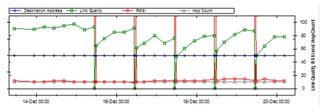
This is expected behavior as we need to turn off the DCAP radio when the cellular modem is active. This is a 30-60 second process that occurs every 12-15 minutes therefore the MDT timing could be just right and it wakes up and transmits during this window and subsequently loses sync. The MDT will however wake up at its next scheduled transmission time (usually one hour) and try again, having stored the prior data point so no MDT data will be lost.
