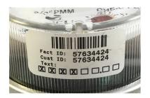
The meter above has eight rotating dials. However, the factory sticker shown on the right says only 4 digits are available to an external reader. Therefore the MDT will report the value of 7. Apply a 100X count factor to get 700 cubic feet, even though the register shows 729.62 cubic feet. Once the register shows 800.00, the MDT will report 8 (or 800 with the 100X count factor applied).
