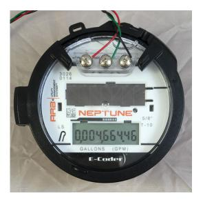
A: The picture here shows a 5/8" E-Coder registers with nine digits total, two digits of which are to the right of the decimal (1/100 of a gallon resolution). Early on Neptune still restricted the encoder output to the upper six digits. Around year 2020 they allowed 3rd party vendors like Tehama to read eight digits.
