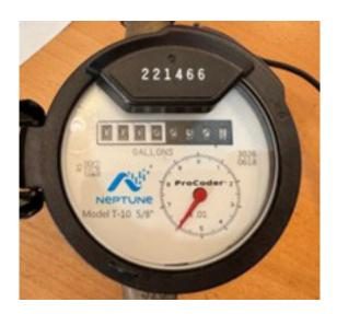
The Neptune ProCoder register pictured above is Neptune's updated mechanical register that displays 8 moving dials. The decimal point is painted between the 7th and 8th dial. Therefore the Count Factor should be set to 0.1 for newer MDTs and to 10 for older MDTs that read only six dials.
