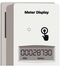
For our Submersible MDT a magnet must be waved across the side of the MDT to activate the internal button. Once a magnet is detected the LED on the front gives feedback that the MDT has been activated.
