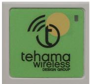
The latest generation MDT, the green circle shows where the hidden button is on the enclosure. An LED to the left gives you feedback when the button is pushed.
