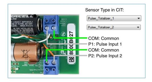
Note that you can swap the Meter connectors and the polarity remains correct.
